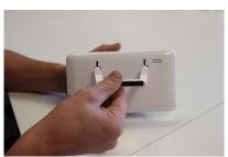
Connect table stand to upper holes on the back of the device and snap into place
