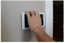
Slide IQ Remote onto wall mount bracket
