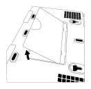
Insert your thumb or finger under the opening on the back cover and firmly pull up to remove.
