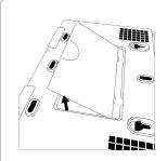
Insert your thumb or finger under the opening on the back cover and firmly pull up to remove. This cover is not needed for wall mount.
