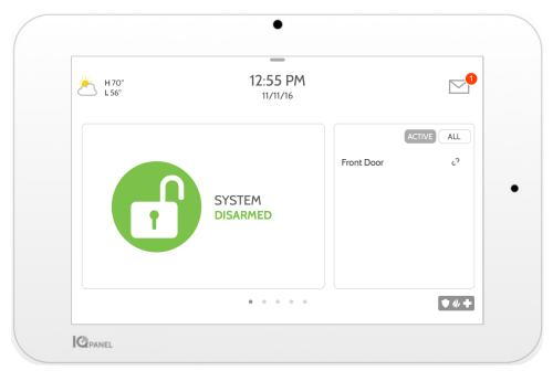
The Qolsys IQ Panel 2 is a 7" touchscreen built with an Android operating system, providing full security and smart home functionality in an easy to use interface.
