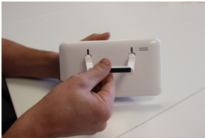
Connect table stand to upper holes on the back of the device and snap into place
