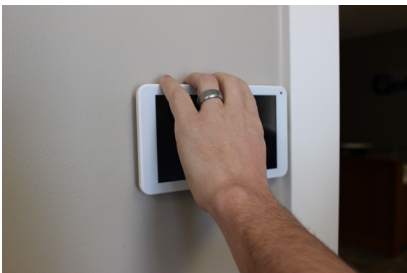
Slide IQ Remote onto wall mount bracket
