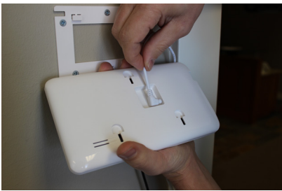
Connect power supply to the back
