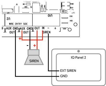
**Optional** Siren Relay wiring using 12v (+) and IQ Panel (GEN1) "Buzzer" output
