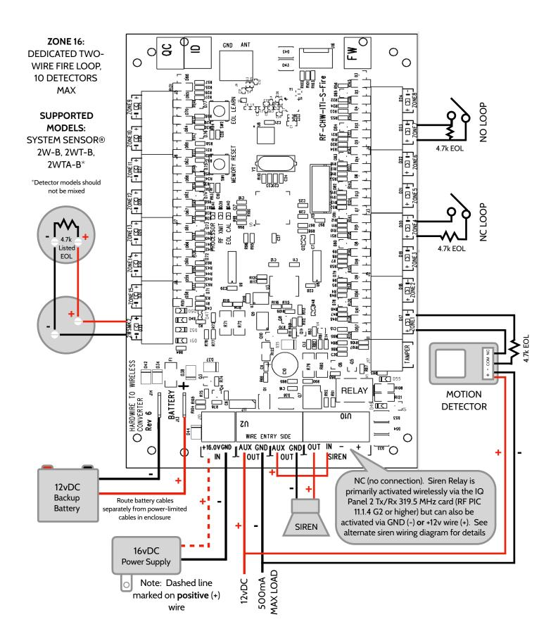
**Optional** Siren Relay wiring using GND (-) and IQ Panel 2 "EXT Siren" output
