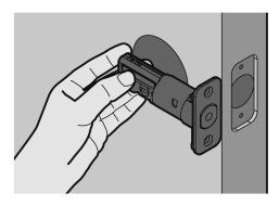
a. If the slotted hole is centered in the door hole, no adjustment is required. Proceed to the next step.
