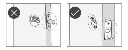
1. Hold the latch in front of the door hole, with the latch face flush against the door edge.
