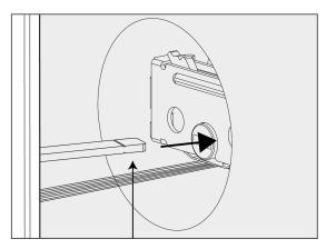
3. Route the cable through the hole in the mounting plate.
