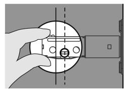
c. Rotate and pull the latch to extend the latch. Adjust so that the slotted hole is centered.
