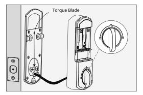
3. Test the lock by rotating the thumb turn to make sure the bolt can extend and retract smoothly.
