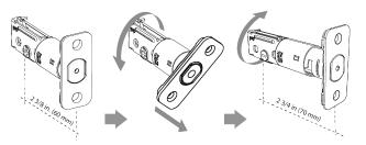
2. Install the latch and use a Philips head screwdriver to secure the latch with two latch screws. Make sure to install the latch according to the UP mark on the latch.
