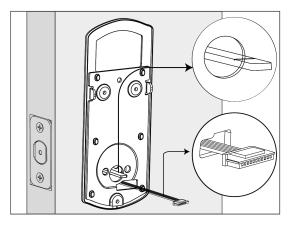
4. Secure the mounting plate to the exterior assembly with two screws.
