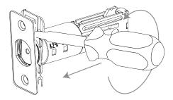
3. Remove the rectangular faceplate. Rotate it counterclockwise and pull.
