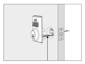
2. Insert the torque blade into the slotted hole on the latch.
