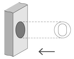
2. If a round drive-in collar is required, remove the rectangular faceplate from the latch with a flat head screwdriver wedged between the faceplate and the faceplate clip.
