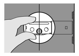
b. If the slotted hole is not centered in the door hole, you need to make adjustments.
