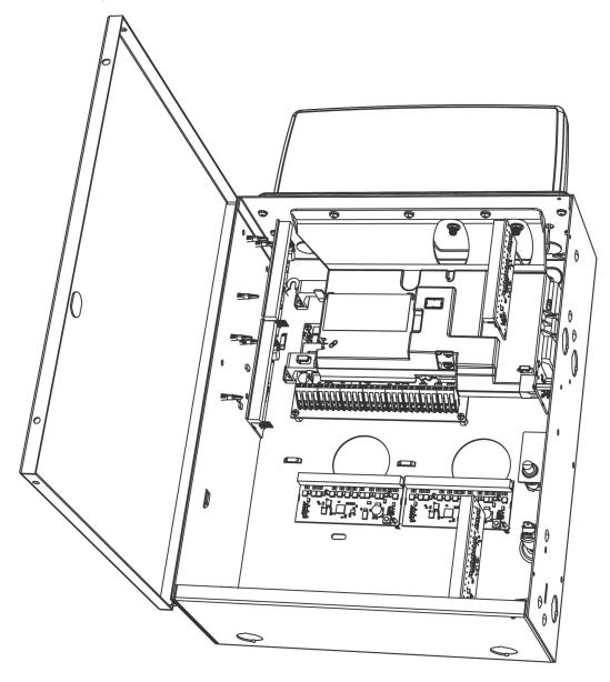
Figure 15: Installing modules in the IQ Pro P
