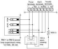
The type of smoke detector must be latching. To reset the smoke detector, refer to the panel installation manual. Note: To locate smoke detectors, refer to the system installation manual and smoke detector installation manual.
