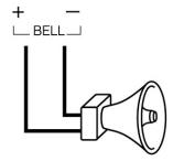
Observe polarity when connecting polarized sirens or bells.
