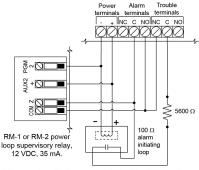
The type of smoke detector must be latching. To reset the smoke detector, refer to the panel installation manual **Note:** To locate smoke detectors, refer to the system installation manual and smoke detector installation manual.
