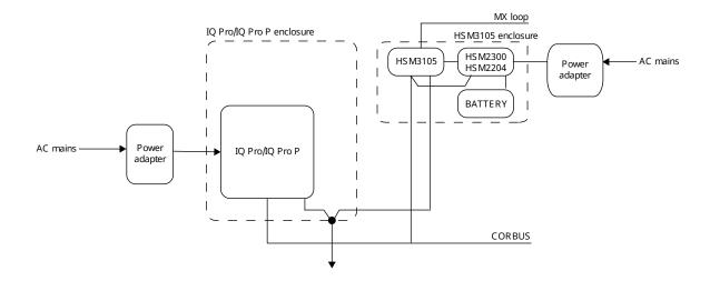
Figure 21: High power mode - wiring diagram
