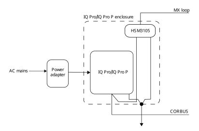
Figure 19: Low power mode - external mount
