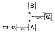
Module (A) is wired correctly as it is within 1000 ft / 305 m of the panel, in wire distance. Module (B) is wired correctly as it is within 1000 ft / 305 m of the panel, in wire distance. Module (C) is NOT wired correctly as it is farther than 1000 ft / 305 m from the panel. For models that require more than 1000 ft / 305 m from the main panel, a power supply/Corbus extender can be used.
