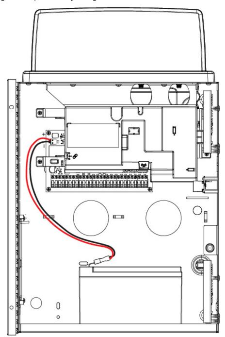
(1) **Note:** You must maintain a minimum separation of 6.4 mm (0.25 in.) at all points between non-power limited battery wiring and all other power limited wiring connections. Do not route any wiring over circuit boards. You must maintain a minimum separation of 25.4 mm (1 in.) between all wiring and the PCB.
