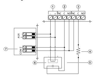
Figure 8: 4-wire smoke and heat detector wiring
