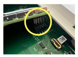
Match the pins on the bottom of the IQ Card to the terminal on the IQ Panel.
