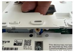
Once the screw has been loosened, pull the backplate away from the panel to remove.
