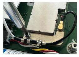
Install and tighten the provided locking screw to secure the IQ Card into place. Ensure the antenna remains connected and does not interfere with the battery.
