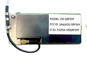
The IQ Card-319 can be installed in to "Slot 3" of your IQ Panel 4, IQ4 Hub or IQ4 NS to enable support of approved S-Line & legacy 319.5 MHz SRF sensors.
