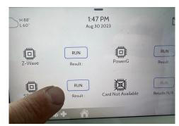
Run the "SRF" test. Allow up to 2 min for the panel to successfully test the radio in the new IQ Card. If test fails, reboot the panel and try again.
