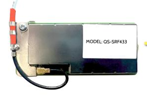
The IQ Card-433 can be installed in to "Slot 3" of your IQ Panel 4, IQ4 Hub or IQ4 NS to enable support of approved legacy 433 MHz SRF sensors.
