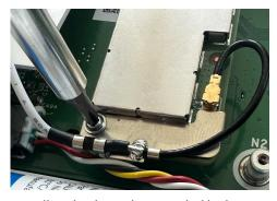
Install and tighten the provided locking screw to secure the IQ Card into place. Ensure the antenna remains connected and does not interfere with the battery.
