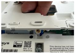
Once the screw has been loosened, pull the backplate away from the panel to remove.
