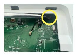
Make sure the PowerG antenna jumper is connected to the main motherboard.
