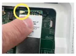
Push the IQ Card firmly into place. Connect the PowerG antenna jumper to the daughter card.
