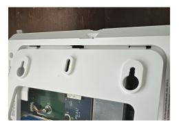
Replace the back cover, top tabs first. Press down on the bottom and tighten the retaining screw.
