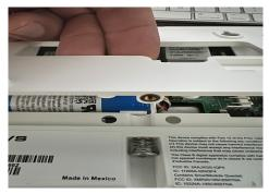
Once the screw has been loosened, pull the back plate away from the panel towards the bottom to remove.
