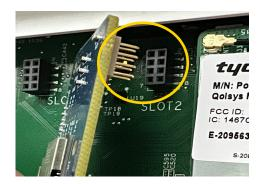
Match the pins on the bottom of the IQ Card-Zigbee to the terminal on the IQ Panel.
