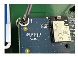
Install and tighten the provided locking screw to secure the IQ Card-Zigbee into place.
