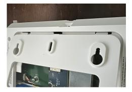
Replace the back cover, top tabs in first. Press down on the bottom and tighten retaining screw.
