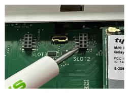
Locate the free card slot to the left of the already installed Power G card (Slot 2).
