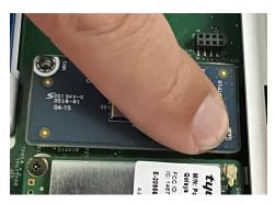
Push the IQ Card-Zigbee into place with your finger over the terminal connection, to avoid seating the card incorrectly or bending any pins.
