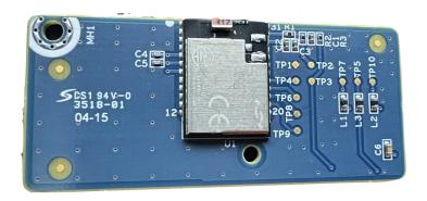
The IQ Card-Zigbee is easily installed in your IQ Panel. This enables support for Zigbee Smart Devices.
