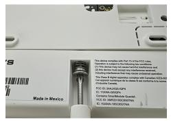
From the bottom of the panel, find the retaining screw. Loosen completely, the screw will not fall out.
